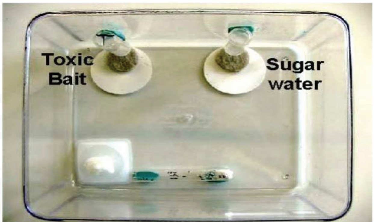
Figure 3. No-choice test experimental setup (Adapted from Warner (2003)).
